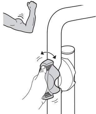
**EN Check the tension.** After a period of use, it may be necessary to check the tension in the knob. Tighten the hexagonal screw half a turn and check that there is greater resistance in the knob when you turn it. **NOTE:** The knob should always be in the tensioned setting.
